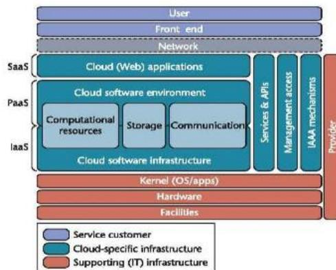
Fig. 1. The cloud reference architecture.
